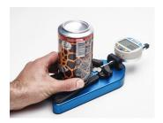
Measure the seam thickness. It is the most important parameter to secure your product.
