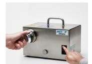
Cut the can with the seam saw in order to observe the inside of the seam.
