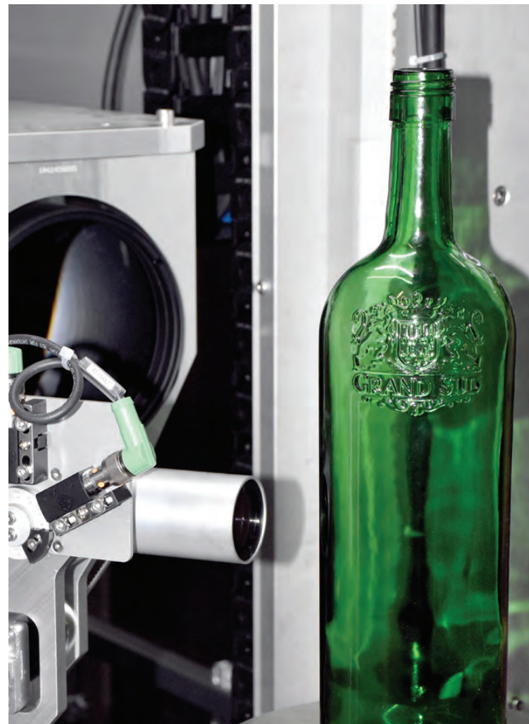
wall thickness measuring station
